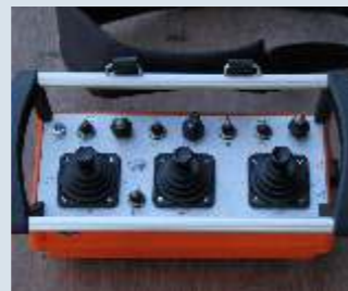
Operator friendly radio remote control along with the option to switch over either to fast/slow boom operation
