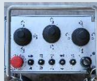
Additional back up cable remote with 24 V electric system
