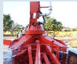
Boom Pedestal with high Power Slew motor which can rotate in a 370 Deg slew range
