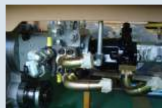
PTO assembly derives power from the truck engine to operate
